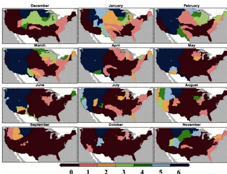
Figure from Shukla & Lettenmaier, (HESSD 2011): Plot of the maximum lead (in months) at which Initial Hydrological Conditions dominate over Climate forecast Skill, for 6-month cumulative runoff forecasts, initialized on the beginning of each month.
