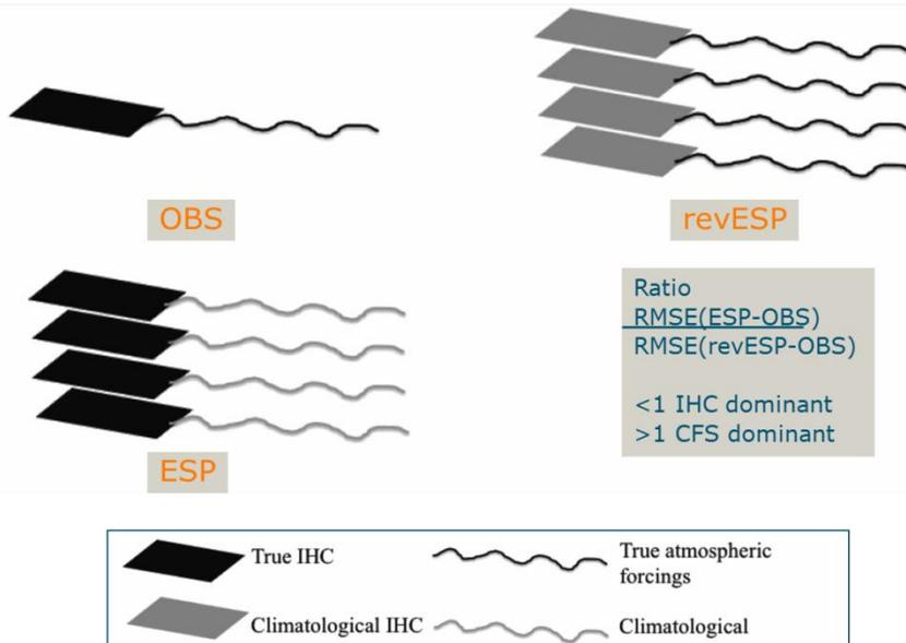
Figure from Shukla & Lettenmaier, (HESSD 2011): schematics of analysing influence of Initial Hydrological Conditions vs Climate forecast Skill on runoff forecasts.
