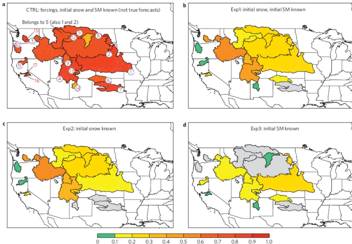
Figure from Koster et al. (2010): Streamflow skill levels in the Western United States achieved in the simulation experiments, plotted by basin. Skill is measured as the square of the correlation coefficient ( $r^2$ ) between MAMJJ total streamflows from simulations and corresponding (naturalized) measurements.
