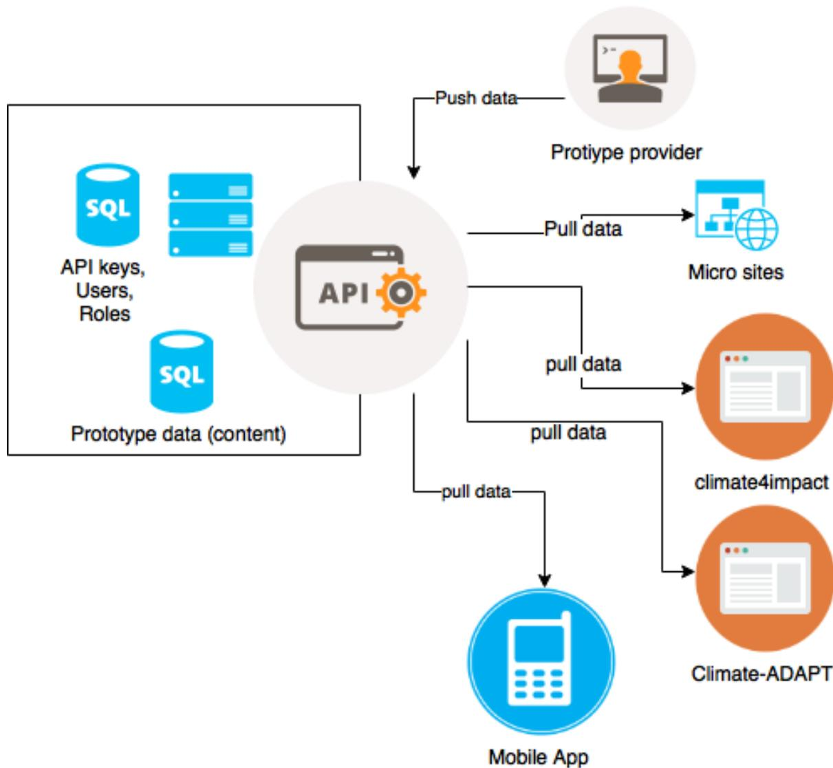
*Figure 1: Schematic of the interactions that the API should support*
